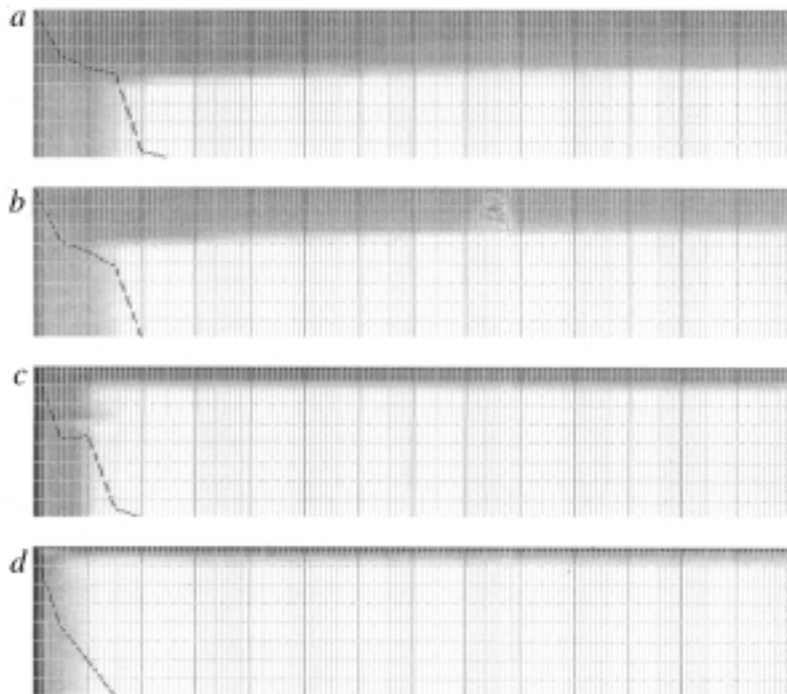
Fig. 4. Distribution of the impregnating fluid in pine railway cross-ties: a) polymer particles are absent; b) 2%; c) 6%; d) 10%.
